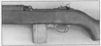
The selector switch next to the receiver above the magazine marks this carbine as an M2. In all other ways the M2 was an exact functional equivalent of the M1 Carbine. Note the 15-round magazine. (below) An M1 Carbine (near) and an M2 Carbine side by side. Only the selector switch and round bolt give away the M2.
